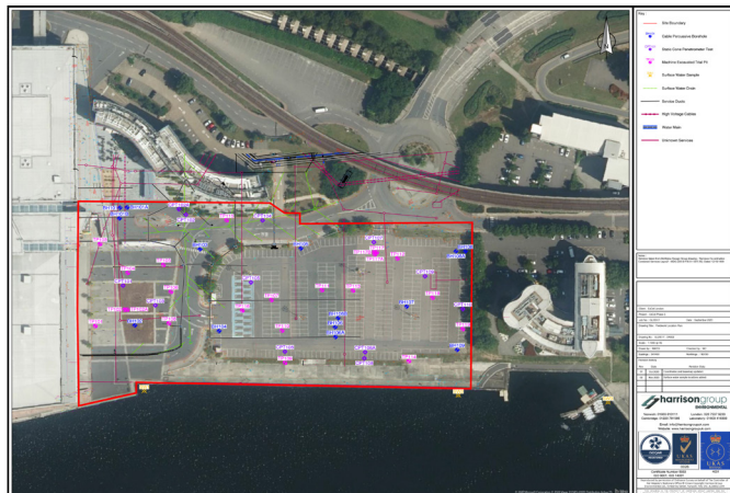
Site plan showing intrusive investigation positions
