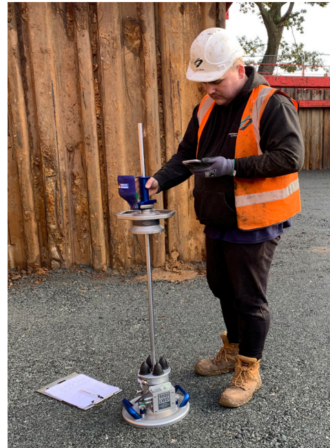
LWD site set-up
