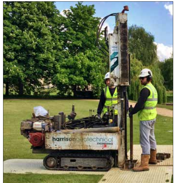
Dynamic sampling and penetration testing rig
